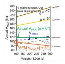
**5.5.** As shown in the adjacent chart, actual  $V_{MCA}$  increases above  $V_{2MIN}$ , if the favorable bank (for this sample airplane 3°) is not maintained and the wings are kept level, except at weights above 240,000 lb.
