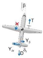
thrust (T) during the remainder of the flight. The rudder generated side force ( $Y_{\delta r}$ ) also causes sideward displacement, resulting in a sideslip ( $\beta$ ). This sideslip, in turn, results in an opposite side force due to sideslip ( $Y_{\beta}$ ). When balance of these forces is achieved, sideslip  $\beta$  increases no more. On a DHC-6 Twin Otter,  $\beta$  is up to 14°. This means lots of drag (D) and hence, loss of climb performance.
